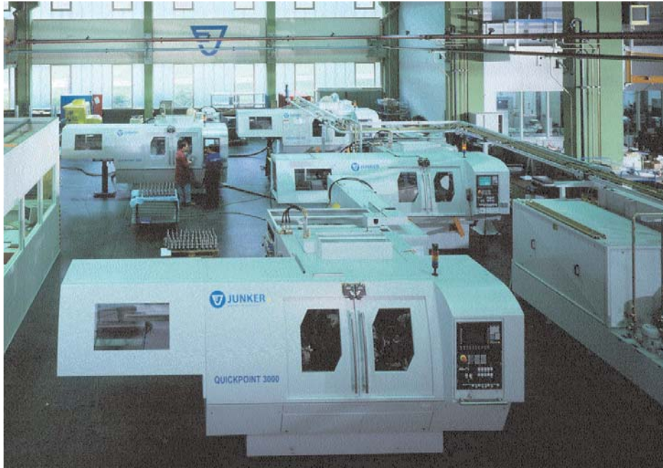
Fig. 1: Finish grinding line for the complete grinding of gear shafts in a single clamping
