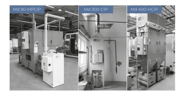
The mechanical particle filters for dust from LTA Lufttechnik are used to collect and remove dust and smoke of any kind. The filtration systems are used for simple industrial applications, but equally for complex industrial requirements and filtrations with special customer specifications. Cartridge and pocket filters are available for cleaning harmful particles.
