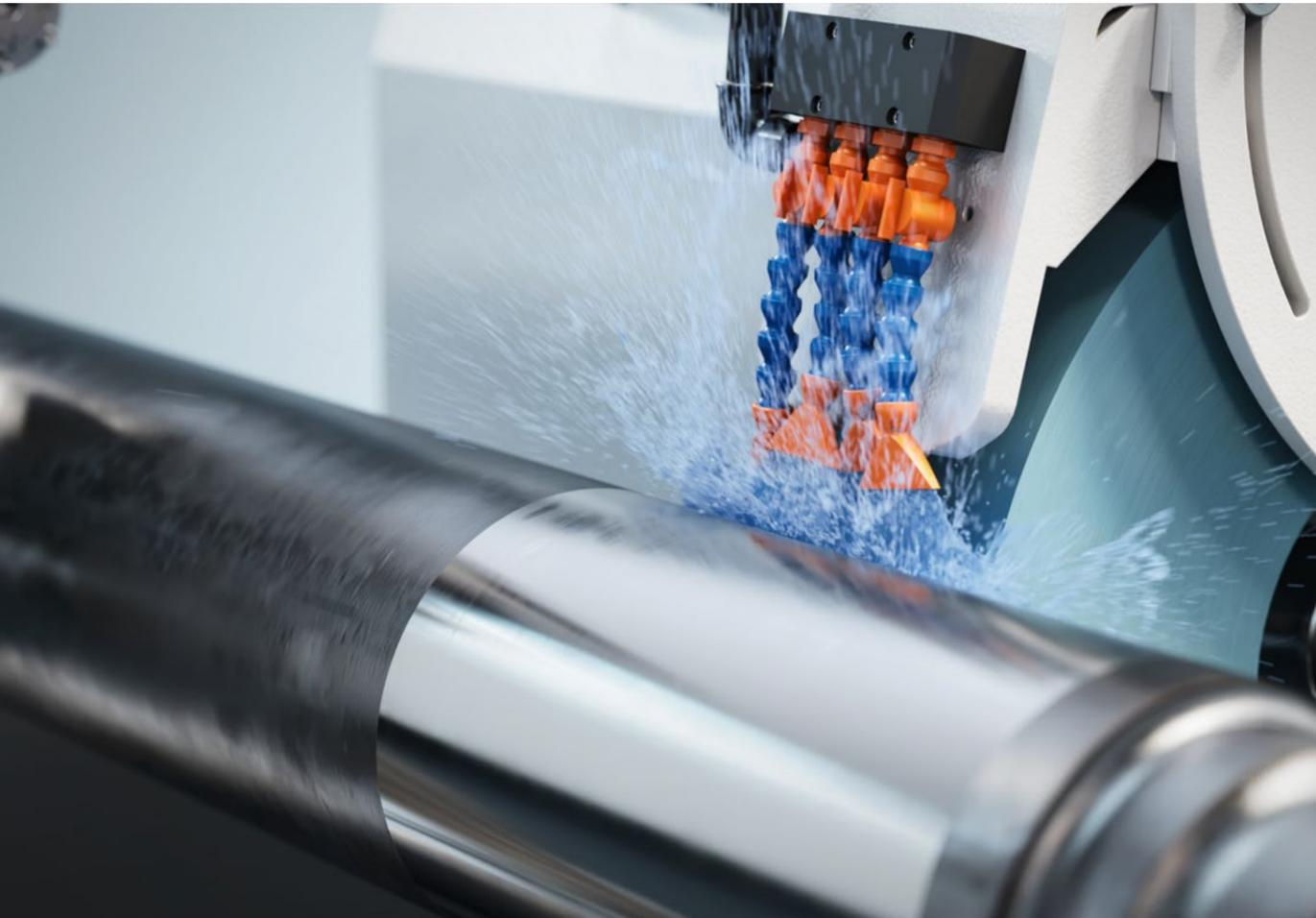
Up to 5.000 mm long and a weight of several tons – the KARGO series tirelessly masters grinding shafts of this size.
