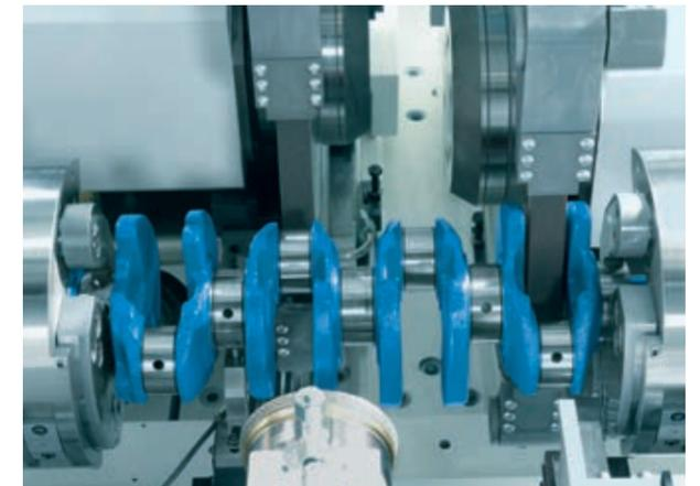
Grinding station 2: Grinding of pin bearings
