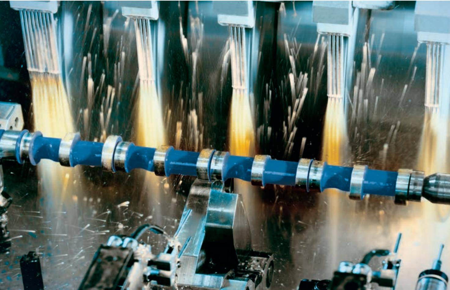
The JUCENTER CBN high-speed grinding machine combines mutually complementary grinding possibilities under one hood. Instead of lining up individual grinding machines for different grinding tasks, both grinding processes take place in two separate clamping set-ups on one machine. The result: highly efficient grinding – all with top precision.
