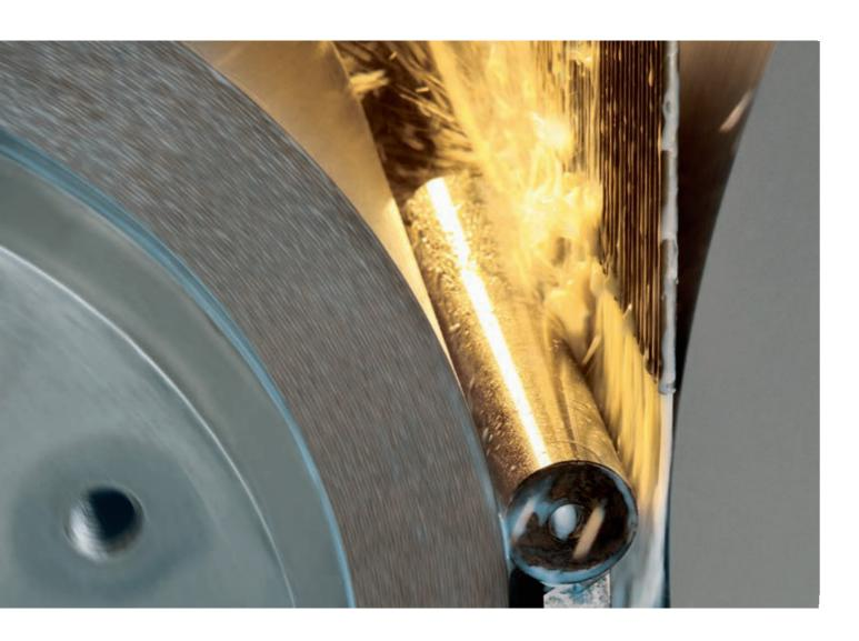
JUPITER series centerless grinding machines offer substantial production benefits: The patented CNC height adjustment of the support blade minimizes tooling times, automatic adjustment of the grinding gap geometry optimizes the grinding process and the inclined bed guarantees maximum dimensional precision. Depending on the application, corundum, CBN or diamond is used as an abrasive.
