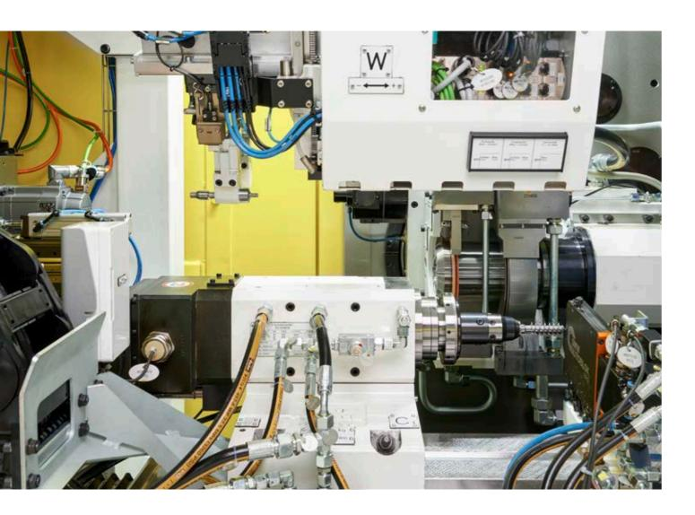
The JUTWIST 2000 high-speed grinding machine establishes worm shaft profiles from blank. The worm shafts are used, for example, in the automotive industry and in general mechanical engineering, where they are used for transmission and power transmission, and are fitted in various steering systems, servomotors and parking brakes, for example. The production process can be easily transferred to other, geometrically similar workpieces.
