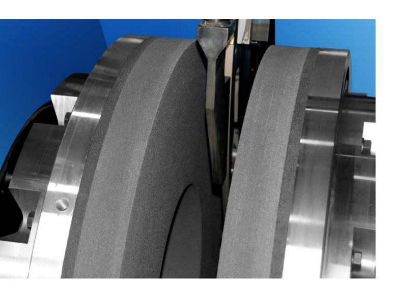
With SATURN double-wheel surface grinding, two vertical grinding wheels grind the workpiece simultaneously at its parallel end faces. With the through-feed grinding process, the grinding wheels are positioned slightly conically to each other so that the workpiece guided through the grinding zone has not reached its final dimension until it exits.
