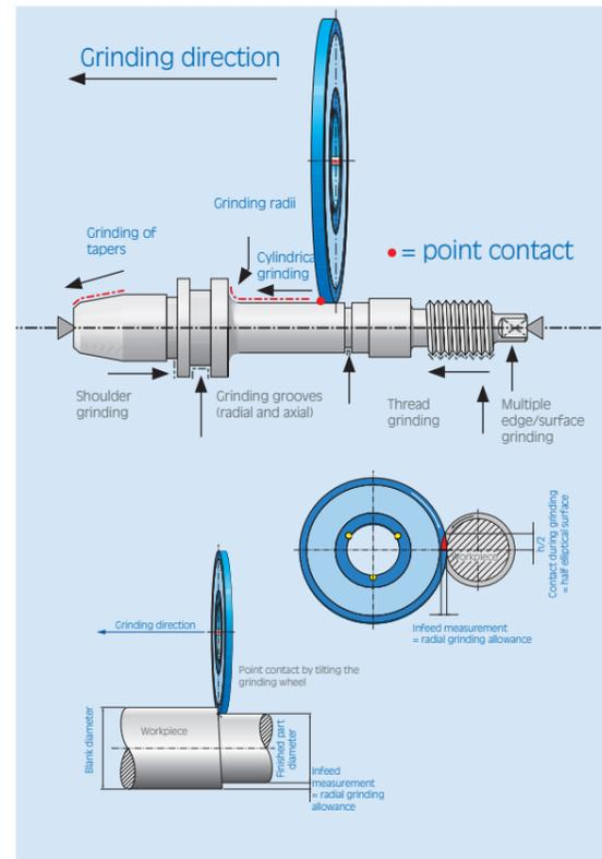
The standard QUICKPOINT grinding operations are shoulders, tapers, chamfers and grooves. Thread grinding and multiple edge and face grinding can be additionally integrated.
